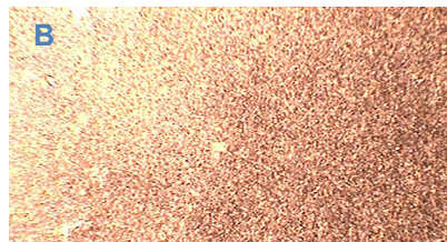
Figure 2: Free BPO (A) and SS BPO (B) dispersed into identical lotion bases (5% BPO) at 42°C. Photographs taken at 100x magnification to show the particle sizes.
