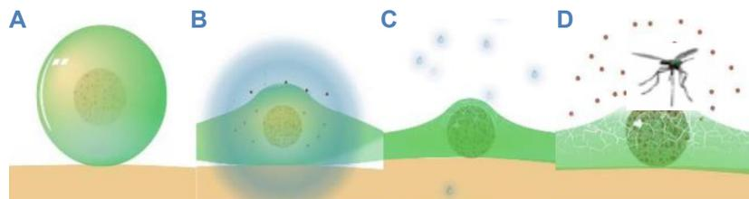
Figure 2: Description of HydroSal<sup>®</sup> changes: (A) the structure in water formula, (B) after application on a surface, the system dries out, turning flat like a film, (C) the dry product is invisible, 1µ or less in thickness. The natural antiseptics are trapped within the polymers, (D) when exposed to water, the water disturbs the polymer to expose the functional ingredients to the environment.
